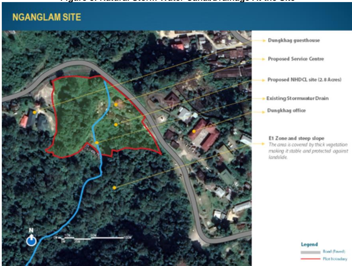
Figure 8: Natural Storm Water Canal/Drainage At the Site
